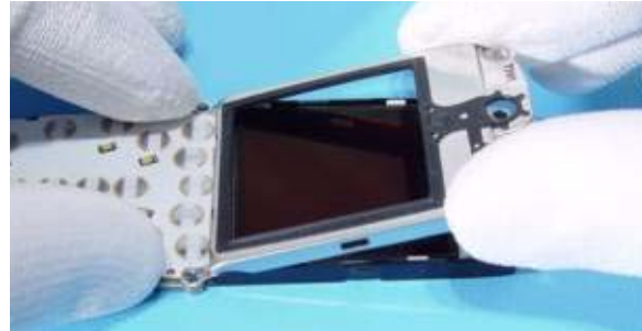
8. The Display Shield is hooked at the bottom edge.
