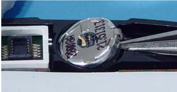
5. The Earpiece is adhered with double-sided adhesive tape. Use new tape when mounting the Speaker .
