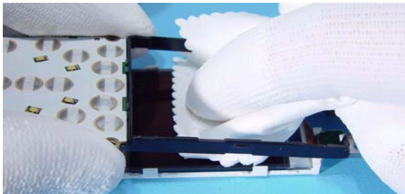
9. Press the LCD off of the LCD Frame . Use a clean cloth as shown above.
